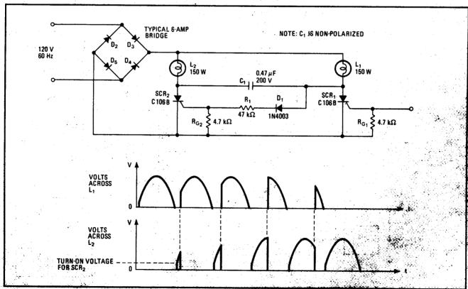
Parts miser. Compliamentary lighting control fades one lamp out while bringing up the other one, with lawer parts than conventional controls use. Waveforms are segments of successive half-cycles of a full-rectified sine wave as control signature.
